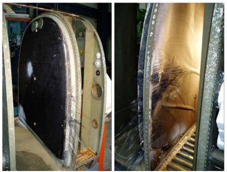
Figure 10: General views to the bulkhead after the residual static test
